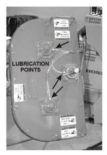
Figure 51. Lubrication Points
